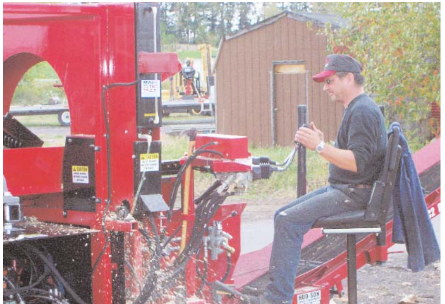
Operator Station w/seat operates with joy stick and push button controls.
