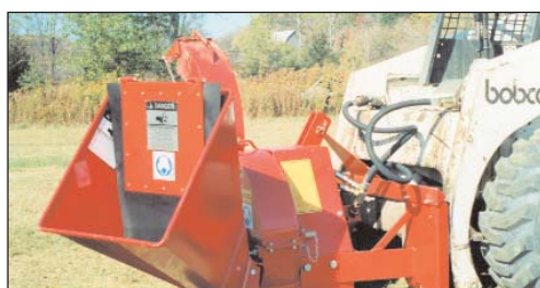
SKID STEER MOUNTED CHIPPER: FOR CH140 HMD/F and CH 140 HMD HF Models Only. Many models are available to suit any customer requirement.
