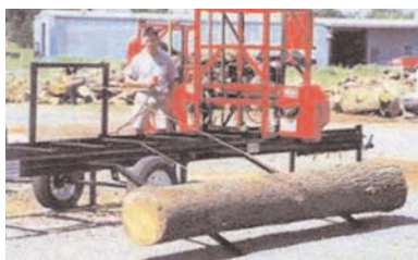
Cable Log Loader & Turner Includes 2500 pound winch and 2 ramps
