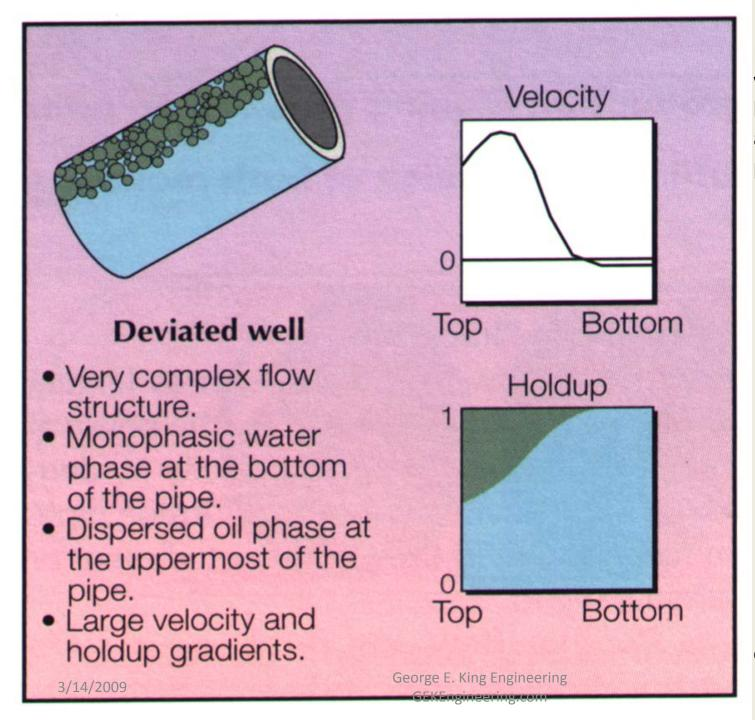
Note the flow velocity difference between the top and bottom of the pipe.
