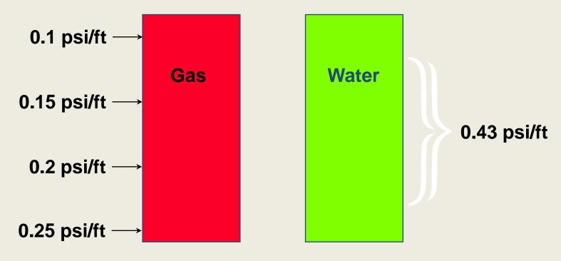
The compressibility of the gas, and the energy stored by that compression, is a key to the flowing energy of the system.
