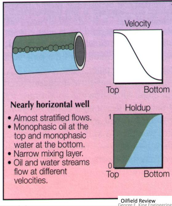
Flow in highly deviated wells is much harder to predict than flow in near vertical wells. In near vertical wells, hindered setting keeps the liquids, solids and gas mixed and all moving upward as long as the gas rate is sufficient to achieve critical rate. In deviated wells however, the lighter fluid separates to the top of the flow channel and the liquids may "percolate" along the bottom in the 30 to 60 degree range, developing liquid holdup and back pressure.
