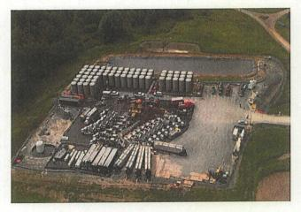
The completions stage takes place in three phases of activity including the hydraulic fracturing described above, "drill out" of the plugs placed in the well during hydraulic fracturing using a small rig, and installation of production tubing (plastic pipe that is used to carry produced natural gas to the surface).
